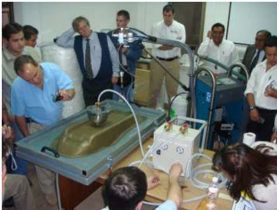
(Stephen Williams of Composite Integration presenting RTM and Vacuum RTM Mold Construction.)
